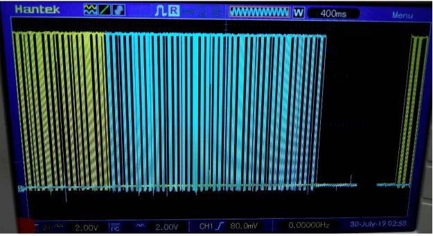
(image achieved by attached channel 1 to Pin 3 of TB3 channel 2 to Pin 4 of TB3)
