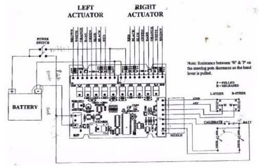
12: Finally, turn off the power switch and wait for 3 seconds. Then turn it on. Now actuator can be controled without reclibration. If that is not happening and error code 6 appears, something is wrong with IC3 (black 8pin chip). The IC3 is in charge of storing calibration data when the power is off. If that happens, replace the IC3. It is an EEPROM named AT93C46D. Replacing IC3 will solve the problem.
