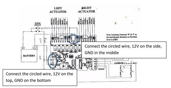
8: Flip the power on. Measure the following voltage of each port in TB3 and TB4. An oscilloscope is preferred in this test. Pin 5 (blue) should be 12V, Pin 6 & 7 (green and bare) should be ground. Pin 8 (orange) should be 5V and Pin 10 (brown) should be ground. If any of the voltage is not seen, first check if there are any broken traces on the circuit computer board. Then go back to step 2. REG-1A may have to be replaced.
